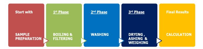
Grind the sample using a grinder (particle size 1mm).
